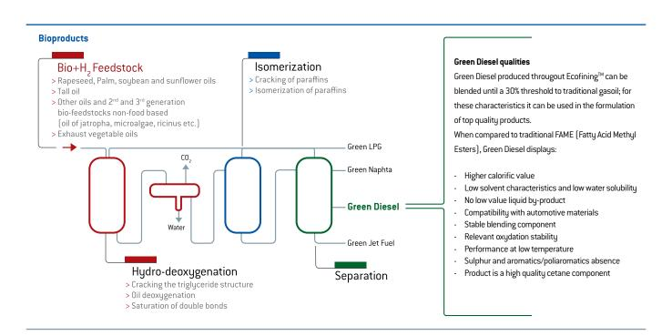
Venice: green refinery entered into production in June 2014, with a production capacity of 360 ktonnes/y. The refinery exploits the proprietary Ecofining™ technology to transform vegetable oil in hydrogenated bio-fuels. A second phase of development is underway. At regime, the production will satisfy approximately half of Eni bio-fuels needs required for being compliant with the EU environmental normative aimed at reducing the CO₂ emission.
