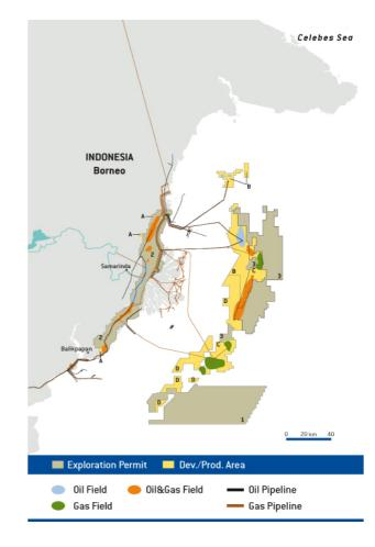
condensate treatment and the construction of a transportation facility to the Bontang liquefaction plant. Start-up is expected in 2016 with a production peak of 80 kBOE/d (41 kBOE/d net to Eni). The Jau project provides for the drilling of production wells and the linkage to onshore plants via pipeline.
