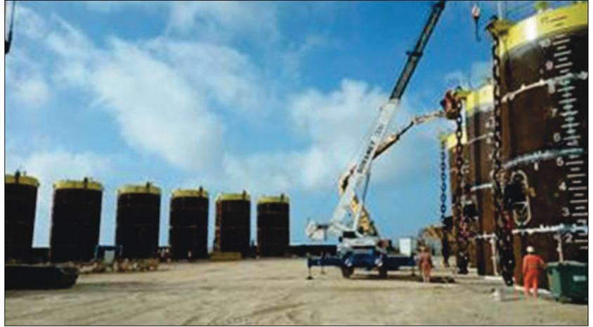
"As part of the Local Content Plan, several fabrication activities have been executed in Angola at Sonamet Yard in Lobito. 9 Suction Piles for the mooring of the FPSO have been completed at Sonamet Yard"
