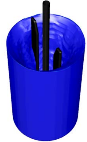
Simulation of free surface of liquid in a stirred reactor
